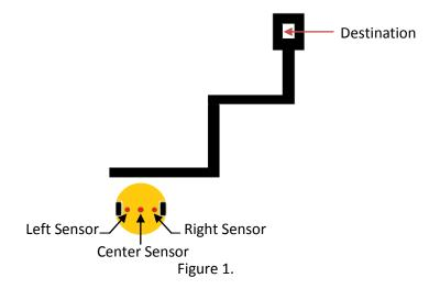
For the test track, your robot is to first move forward until it identifies the line. It should then proceed to orient itself in the proper direction. Next, the robot should follow the line to the final destination. Once the destination is reached the robot should shut down and cease moving.
